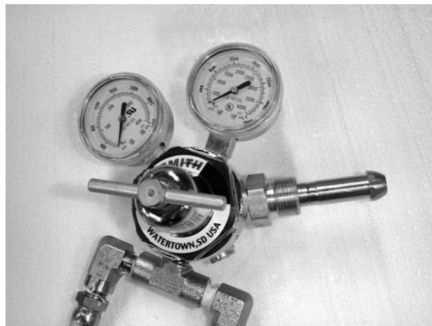
One regulator controls the nitrogen pressure for both chemical tanks. The nitrogen gauge shows the pressure inside the nitrogen tank.
