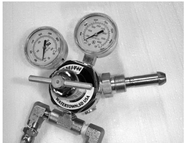
Above are the nitrogen pressure gauges and regulator.
